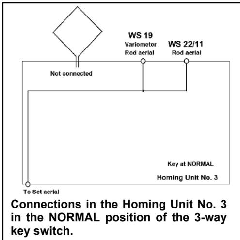
Connections in the Homing Unit No. 3 in the NORMAL position of the 3-way key switch.
