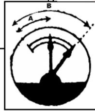
Meter deflection of HOMING 1 -A- and HOMING 2 -B- with the homing sender position at the right hand side.
