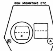
THE REAR FLAP X OF THE CMDR'S CUPOLA (WHICH ROTATES) CAN BE LOCKED IN A POSITION 70° TO HORIZONTAL. METAL THICKNESS IS LESS THAN 1/4"
