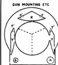
TURRET FLAP Y. ABOUT 10° TO HORIZONTAL WHEN OPEN-FLAPS WILL ROTATE ON RING. CAN BE MOUNTED AT Y; METAL THICKNESS BEING APPROX 15 C/M
