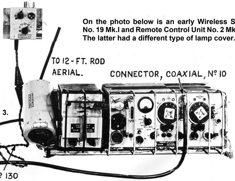
On the photo below is an early Wireless Set No. 19 Mk.I and Remote Control Unit No. 2 Mk.I. The latter had a different type of lamp cover.
