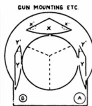
TURRET FLAP Y. ABOUT 10° TO HORIZONTAL WHEN OPEN-FLAPS WILL ROTATE ON RING. CAN BE MOUNTED AT Y; METAL THICKNESS BEING APPROX 15 C/M
