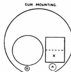
THE TURRET FLAP X CAN BE LOCKED IN THE VERTICAL POSITION AND THE CLAMP FIXED TO THE TOP EDGE. THE METAL IS APPROX 20 M/M THICK.
